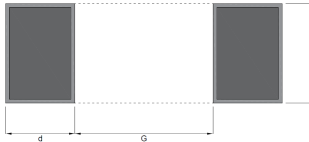
Figure 3.3. A warehouse module for row storage without equipment with parallel arrangement of palletised LU
